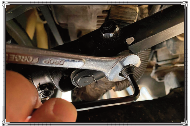
Our Toyota is equipped with a Borgeson steering shaft. We removed the set screws and the long pin/screw that goes all the way through the unit. We then slid the steering shaft off of the power steering box sector shaft.
