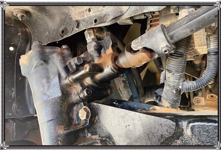
This seriously leaking steering box is the main reason we opted to make a few upgrades on the truck. The old steering box got us off the trail and home safely on its last outing, but continued use in this condition would be asking for trouble.
