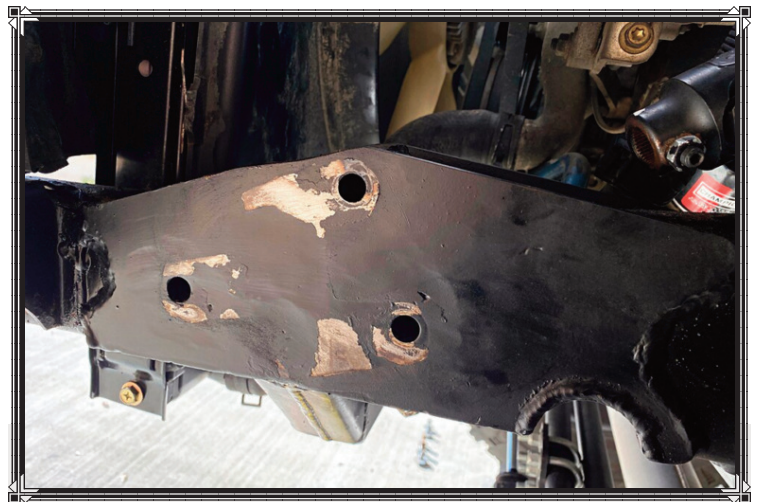
With the steering box removed it was a good time to completely flush and clean all of the caked-on steering fluid from the frame and box mounting area.
