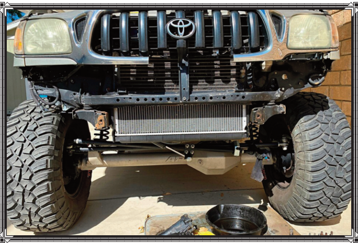
To make things easier for the steering box removal and to allow assessment of the frame and mounting hardware, we removed the Tacoma's aftermarket front bumper.
