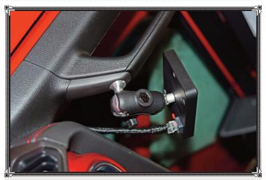
Control of the sPOD 8-Circuit Source SE and the Baja Designs XL80 LED light is accessed through the system's touchscreen. We mounted ours onto the Jeep Gladiator's A-pillar, with a Ram Mounts Double Socket Arm securing it to a Carolina Metal Masters A-pillar Ball Mount attached to thread holes accessed under the plastic A-pillar cover.
