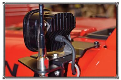
With the driver-side (pictured) and passengerside Baja Designs XL80 LED lights mounted to the Mopar A-Pillar Brackets, plugged in and ready to go (along with our HAM and CB antennas sharing the Mopar mount platforms), we were ready for another testdrive.
