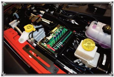
On board to manage a multitude of electrics that are planned our currently installed on this Jeep was an sPOD 8-Circuit Source SE w/Touchscreen system. The wiring from the Baja Designs XL80 lights were routed into the engine compartment and fed into the circuit board of the sPOD system.
