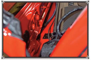
The Ethernet cable connecting the sPOD Source SE circuit boards to the touchscreen was strung through the cowl and then up through the bottom of the Gladiator's fold-down windshield.
