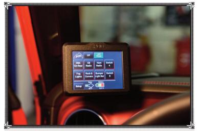
The controls to the new Baja Designs XL80 LED lights were, quite literally, at our fingertips. Switching them on and off is as simple as tapping the screen, but the sPOD 8-Circuit Source SE touchscreen can also be used to make the lights strobe, flash, or come on momentarily, as well and allowing you to take advantage of the dimming (20 percent) feature of the Baja Designs XL80 LED lights.
