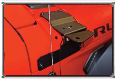
The broad upper platform and extended lower support of the Mopar A-pillar bracket design create a perfect station for our new Baja Designs XL80 LED lights.
