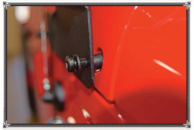
Kit-supplied spacers keep the A-pillar light bracket off the sheetmetal and help to create a sturdy connection between the bracket and the body panel.
