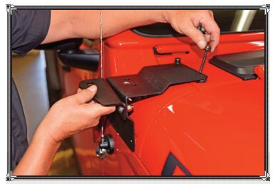
All-new replacement hardware for the cowl corners comes with the Mopar bracket kit. A ratchet with a T-30 for the top two bolts and a T-40 for the bottom two bolts gets the job done quickly.
