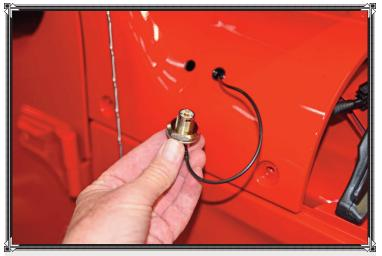
The four factory bolts holding each of the cowl corners were removed. Then very carefully drilling with a pilot drill first, we made two 1/2-inch holes in each to thread the wiring through and used locking plastic grommets to protect the wiring. Our plan was to share space on the Mopar A-pillar lamp brackets for the Jeep's Ham and CB antennas, so they were wired up first.
