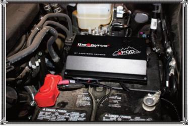
With the Source SE bolted to the fuse box cover, it was conveniently located on the driver side of the truck, enabling it to be aligned to the firewall pass-through grommet and battery.
