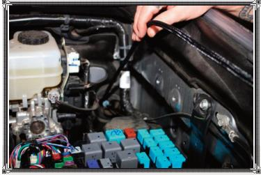
To connect the HD Switch Panel to the Source SE unit, a 10-footlong Ethernet cable is included and runs through the firewall grommet on the driver side.
