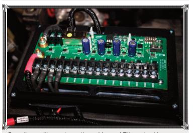
Once the positive and negative cables and Ethernet cable are connected, it's time to plug in a few accessories. The Source SE features eight circuits rated at 30 amps at 12.5 VDC per circuit, and are user-friendly terminally blocked? for attaching accessories. The accessory wiring pushes through a rubber membrane to help keep the Source SE box free of dust.
