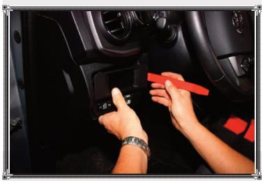
After sampling various locations to mount the HD Switch Panel in our Tacoma cab, we ended up mounting it to the open 3x2-inch cubby that sits to the left of the steering column.
