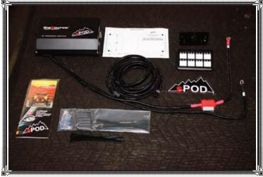
The Universal 8 Circuit Source SE System with HD Switch Panel includes all mounting bracketry and necessary hardware to install an sPOD into any truck, car, RV, UTV, boat, or in our case, a '17 Toyota Tacoma 4x4 TRD Off-Road. Fuses are a thing of the past with the Source SE system, and have been replaced with current-sensing MOSFET's controlled by a microprocessor.
