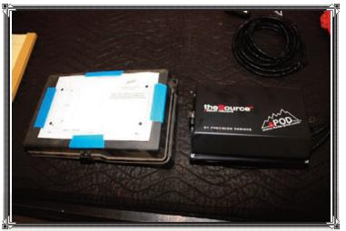
The Source SE fits nicely on the top of the Taco's fuse box. A handy template helped line up the supplied mounting bracket.
