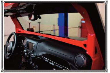
The EVO MFG Dash Cross Bar should be installed before both A-pillar support bars are installed. This makes the job a lot easier. All the hardware should be left loose enough to make small fitment adjustments prior to tightening down the a-pillar supports, connector plates, and dash cross bar.
