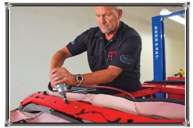
The last piece in our Jeep Wrangler JK sport cage upgrade was bolting the EVO MFG Chromoly Sport Cage Rear Bar to the EVO B-pillar cross bar and C-pillar cross bar. It mimics the EVO front center bar by splitting the area above the Jeep's rear bench seat in two. Some interior fascia trimming is required to install the EVO sport cage rear bar.
