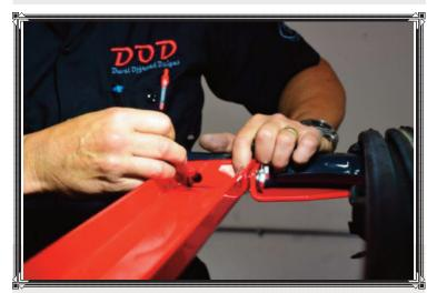
Installation of the EVO MFG Upper Cross Bar was next. The upper cross bar spans the factory tubes above the front doors and is mounted just behind the previously installed connector plates. Some drilling of the factory tubes above the front door is required for installation of the upper cross bar.
