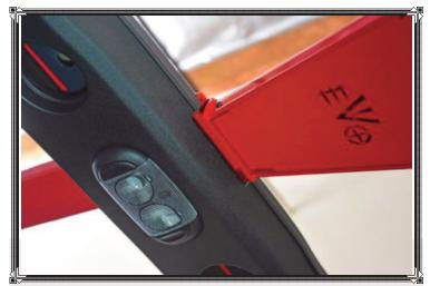
Installation of the EVO MFG Chromoly Sport Cage Kit also requires some trimming of the front of the plastic cover to the factory sound bar. Marks for trimming can be best made by temporarily bolting the sound bar back on to the B-pillar cross bar, then removed again for trimming before final reinstallation.
