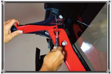
The EVO MFG A-Pillar Support Bar is also connected to the upper factory cage system through kit-supplied EVO MFG Connector Plates.
