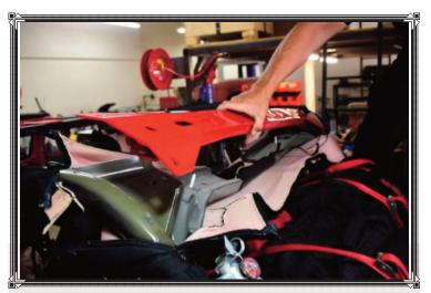
We also ordered the EVO MFG Chromoly C-Pillar Cross Bar (P/N EVO-1168) and EVO Chromoly MFG Sport Cage Rear Bar (P/N EVO-1157). Installation of the EVO MFG C-pillar cross bar requires removal of the factory C-pillar cross bar. That begins with the removal of all the fabric and padding from the factory C-pillar cross bar. The wiring harness must also be loosened from the factory C-pillar cross bar.
