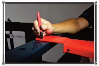
The EVO MFG Center Bar splits the air over the front passenger area and is bolted to the EVO upper cross bar and the factory B-pillar bar; some drilling of the factory B-pillar cross bar is required.
