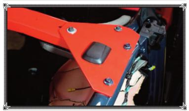
But here's the twist, if you get the EVO MFG Chromoly B-Pillar Cross Bar (P/N EVO-1167) along with the basic Sport Cage kit (as we did), the EVO MFG B-Pillar Cross Bar lays on top of the factory B-pillar cross bar and adds another notch of security and strength. The EVO MFG B-pillar cross bar is attached using the EVO MFG B-Pillar Plates (they double-up the factory B-pillar plates), and the EVO center bar is attached to the EVO B-pillar cross bar in this case—rather than the factory cross bar.
