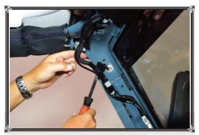
The windshield visors and the plastic panels in the upper corners of the A-pillars on each side of the dash and along the windshield frame must be removed, and the wiring harness needs to be loosened in preparation for the EVO MFG Chromoly Sport Cage (P/N EVO-1156) installation. The plastic panels that fit in the upper corners of the A-frame and windshield have to be trimmed per the installation instructions to accommodate the EVO A-Pillar Support Bars.
