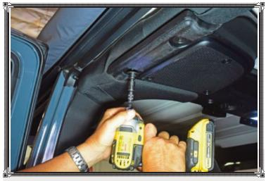
The foam pads on the factory tubes over the front doors have to go (for now), and if you have a sound bar it will also have to be removed to allow for installation of the EVO MFG Upper Cross Bar and Center Bar.
