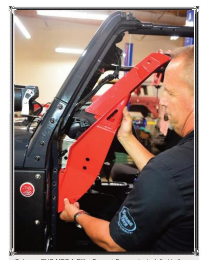
Only one EVO MFG A-Pillar Support Bar can be installed before the EVO MFG Dash Cross Bar is in place. We began with the driver side and maneuvered the A-pillar support bar into place, and then loosely bolted its bottom end.
