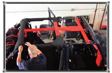
Once all the pieces of the EVO MFG Chromoly Sport Cage kit and the optional EVO Chromoly B-Pillar Cross Bar, EVO Chromoly C-Pillar Cross Bar, and EVO Chromoly Sport Cage Rear Bar were in place and all the hardware was torqued down, the previously removed wiring, padding, and zipped covers could all be reassembled and buttoned up to finish the installation.
