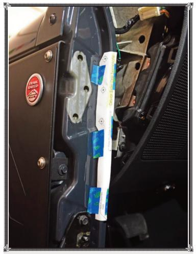
The doors should be removed to make this install easier. The kit includes a template for the three holes that must be drilled in each of the front door sills for the EVO MFG Chromoly Sport Cage A-Pillar Support Bars. The paper template included in the installation instructions shows exactly where to punch and drill the holes.
