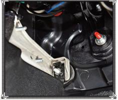
After locating the metal reinforcement plate above the plastic kick panel on the driver side of the Jeep, we tucked the dead pedal kit's backing plate behind the factory reinforcement plate so the backing plate's welded-in 1/4-inch threaded bolts poked through the upper and lower holes in the reinforcement plate closest to the firewall. Now the M.O.R.E. dead pedal and its mounting plate (assembled using kit-supplied hardware) can be bolted up using the 1/4-inch flat washers and nuts in the kit.
