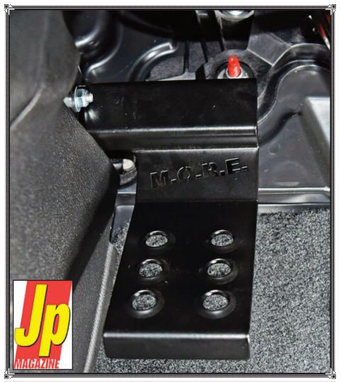
In any vehicle, regardless of transmission type, drivers can use the dead pedal to brace themselves while maneuvering the vehicle, helping to maintain better vehicle control. We picked the M.O.R.E. #DPJL18 for this job, as it was designed specifically for the Jeep JK Wrangler with automatic transmission but also fit perfectly into the automatic-equipped 2020 Jeep JT Gladiator.
