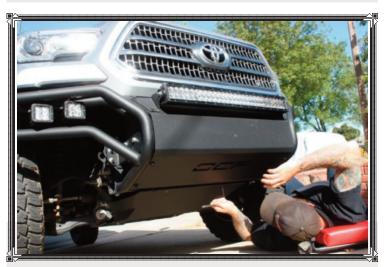
The factory skidplate on the Tacoma is wafer thin and we've already customized it with an obstacle. The OCF skidplate is manufactured with heavy-duty 12-gauge solid steel and it bolts up to the factory location protecting the underbelly from rock rubs.
