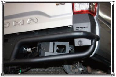
OCF's rear bumper ships in two pieces and bolts up to the factory mounting location. Thick-walled 1.75-inch-diameter tubing and heavy-duty 10-gauge steel mounting brackets are included. Also included are mounting tabs for the factory backup sensors (if factory optioned) and additional reverse lighting.
