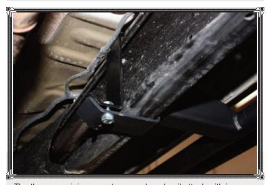
The three remaining mounts on each rock rail attach with inner brackets that wrap around each framerail and are bolted using the supplied hardware. Once torqued to spec, the rock rails are ready to take some serious abuse.
