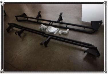
OCF's rock rails are designed as two-piece units and bolt together at the center section. OCF manufactures two rock rail options, a shortbed and longbed version. The rails bolt on, using existing holes and cradles to the frame. With the longbed Tacoma, the wheelbase extends to 140.6 inches, which is a lot of real estate to expose on the rocker panels, so the OCF rock rails have them covered.
