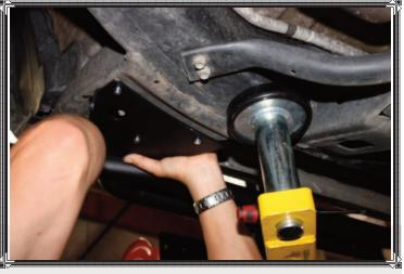
The rock rails attach to four locations on each framerail, ensuring a solid base. The front mount on each rock rail utilizes a stout body pad on each side of the truck, located behind the front wheelwells, with three bolts for a secure connection.
