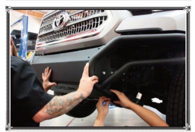
The center section and corners are adjustable, enabling you to line them up to the grill and the trimmed factory plastic cover, below the headlights.
