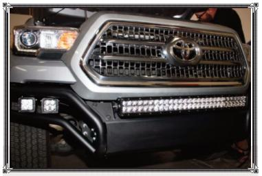
Rigid Industries' 3-inch square Dually LEDs fill the void in the tubular corners, with one spot and one flood on each side. Each Dually puts out 1,568 raw lumens and only draws 1.45 amps. The center section is set up to accept Rigid's 28-inch E-Series LED combo LED lightbar, which puts out a whopping 12,880 raw lumens and only draws 11.16 amps.
