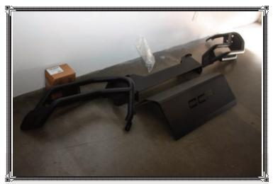
OCF's front modular bumper ships in four pieces, which significantly reduces shipping costs. The tubular corner sections are manufactured from 1.75-inch-thick tubing, along with 10-gauge steel mounting brackets. The 12-gauge steel center section protects vulnerable components.
