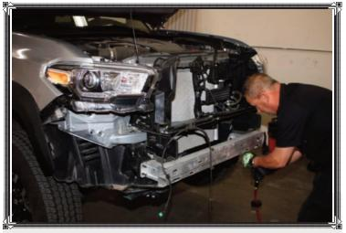
Beginning at the front, we removed the entire factory bumper cover and disconnected the factory fog light wiring. The lower aluminum crossmember unbolts and the factory holes are then utilized for the Off Camber Fabrication (OCF) bumper.
