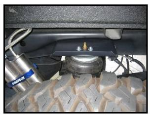
Install air fitting in airbag and attach bag to upper & lower brackets. Repeat bracket and bag installation on opposite side of vehicle.
