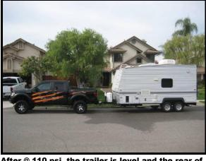
After @ 110 psi, the trailer is level and the rear of the truck is at an acceptable height!
