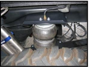
Carefully route air lines to each bag avoiding heat sources and sharp obstructions. When all connections are finalized, inflate system and check for leaks with soapy water.
