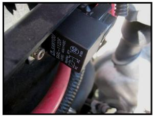
A heavy-duty relay is provided in the kit. We attached it to the side of the battery box, which worked out very well.
