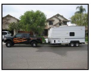
Before, the trailer is noticeably low in the front and the rear of the truck is sagged.
