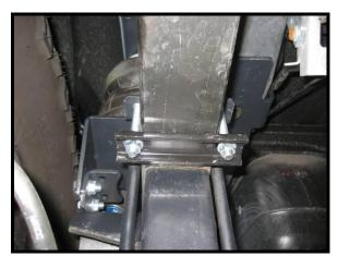
Attach lower spring plate to top of leaf spring with 3/8" carriage bolts and plates as shown. Axle support bracket would normally be adjusted to rest on axle tube, our installation rests on the wing of the modified lift block.
