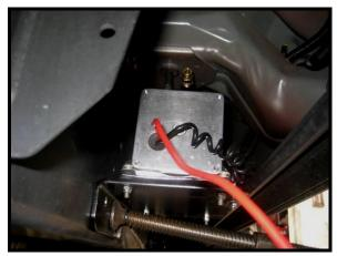
Next, we fabricated a bracket to attach the compressor to the outer passenger frame rail.
