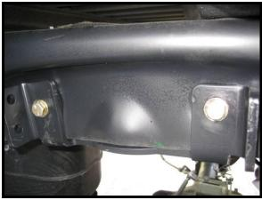
Slide the nut tabs in from the back side of the frame and attach 3/8' bolts loosely.
