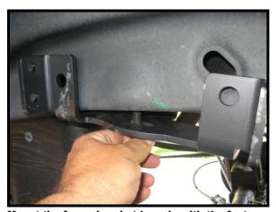
Mount the frame bracket loosely with the factory bump stop bolt. Pay close attention, there are left and right hand specific brackets in the kit and the variations are slight.
