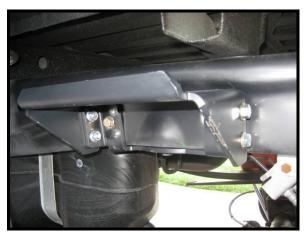
Attach upper bag bracket to frame bracket with 3/8" hardware. Once everything is in place, tighten all hardware.
