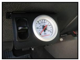
First, a suitable mounting location for the air controls was chosen. Then the air lines and compressor trigger wire were routed into the engine compartment through the firewall. The gauge backlight wires were connected to the factory dash light circuit by tapping in at the back of the headlight switch.
