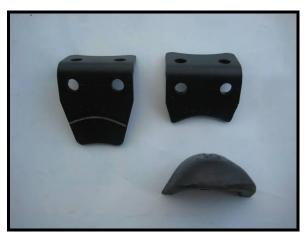
Once the block was cut, we also cut the support bracket to fit the new contact point.
