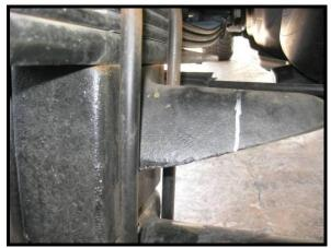
Because our truck has a lift kit, the distance between the leaf spring & axle is increased by the thickness of the lift block. Since the factory bump stop is permanently removed, we decided the raised bump wing on the lift block would make an adequate rest for the bracket that would have normally rested on the axle tube. We marked where the bracket hit to cut the excess off the block since we would be rotating it to the outside of the spring for our installation.
